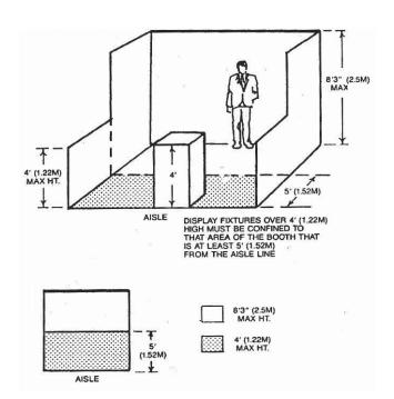
**IMPORTANT:** Space dimensions shown on floor plan are from centerline of booth equipment, such as side rails and/or back drape. Exhibit structures must be constructed to allow sufficient tolerance on each side for this equipment and for utility service at rear of booth.
