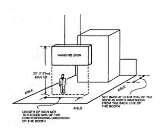
indicating that the structure is built in compliance with the details and specifications set forth on the drawings. (Note: Exhibitors are encouraged to use lightweight materials in the construction of a hanging sign to eliminate excess stress to the facility ceiling structure.)
