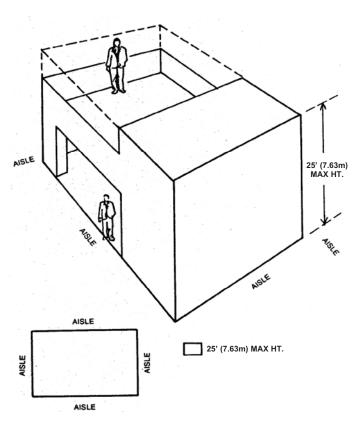
**IMPORTANT**: Exhibitors are cautioned when installing a display with a ceiling or second level to check with the local fire department to insure that their display meets with the necessary fire safety precautions involving smoke alarms, fire extinguishers, sprinkler systems, etc.
