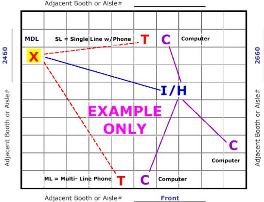
X = Main Distribution Location (MDL) – The originating line(s) for service, whether from overhead, a floor pocket or a column, will be delivered to a "MDL" before being distributed within your booth. Example: Storage area, back of booth, etc. (unless specified, the
