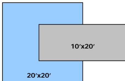
*The amount of covered area in this example is 500 sq. ft. based upon a “Plan-View Perspective”. Although the two elements total 600 sq. ft., the overlapping portion is not considered in the covered area calculations.*
