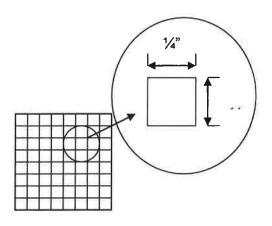
The unobstructed openings in the material must be at least  $\frac{1}{2}$  inch in two directions.
