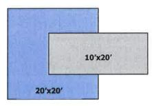
The amount of covered area in this example is 500 sq. ft. based upon a "Plan-View Perspective". Although the two elements total 600 sq. ft., the overlapping portion is not considered in the covered area calculations.
