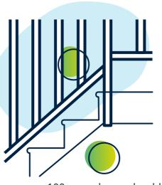
100mm spheres should not pass through
